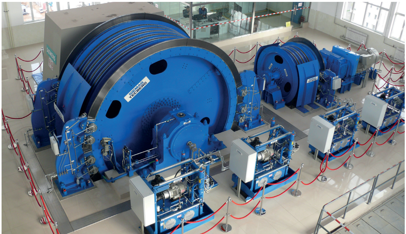
Fig. 2: Reference photo SIEMAG TECBERG 6-rope Koepe hoisting machine installed on tower Copyright 2022 Tianjin SIEMAG TECBERG.
