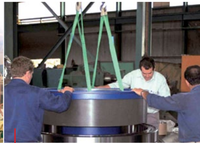
Assembly of the winder in the workshop
